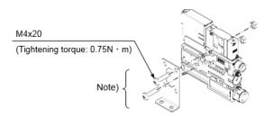
Note) Mounting bracket for single unit (Option) [Nuts and bolts are included.] Part number: ZK2-BK1-A
