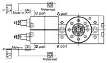
\* The table return position under the power-off state changes depending on the solenoid valve type. Please refer to page 299 for details.
