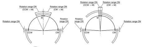
: Operating range of auto switch CCW: Counterclockwise M: Center CW: Clockwise
