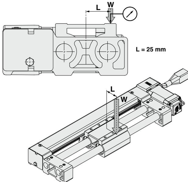
Load center of gravity located at a position offset when L = 25 mm
