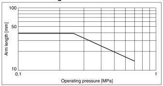
When the arm length is 35 mm, the pressure should be 0.28 MPa or less.
