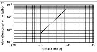
When the arm's moment of inertia is 5.2 x 10-5 kg·m2, set the rotation time required for a  $90^{\circ}$  rotation to 0.1 s or more.
