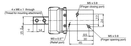
\*1 The dust cover features an internal sealed construction which prevents internal pressure fluctuations. In addition, there is a relief port which allows for the release of the small amounts of air leaked from the air gripper.
