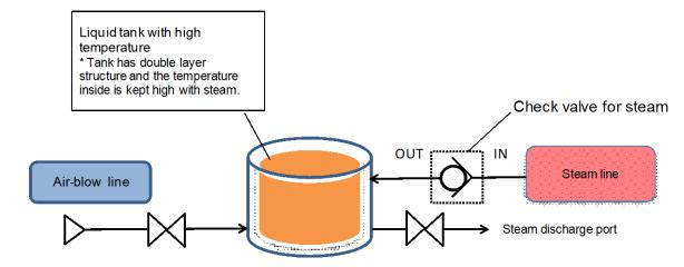
Application example 2: Steam line to be used for rubber molding (vulcanizer), such as tires
