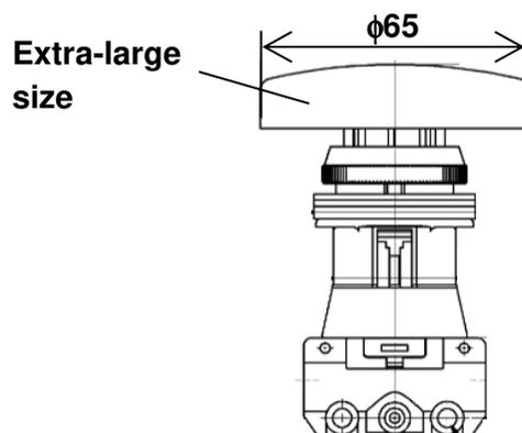
The button can be pushed with a palm, which reduces fatigue.
