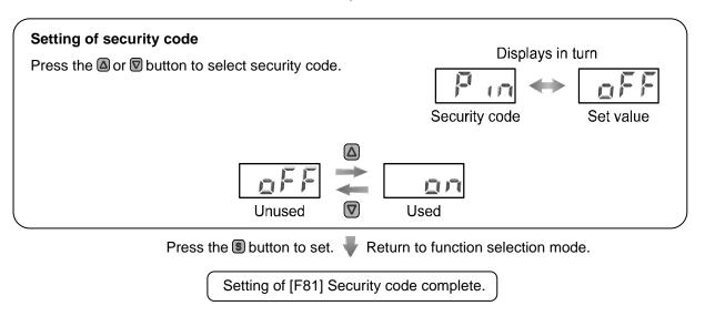
If the security code is used, it becomes necessary to enter the security code to release the key lock. The security code number can be set to a different value by an operator. The default setting is "000".
