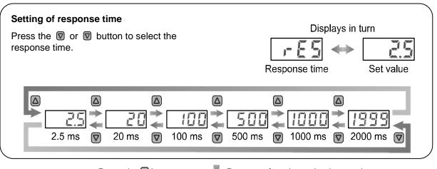
Press the S button to set.  $\P$  Return to function selection mode.
