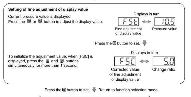
Setting of [F 6] Fine adjustment of display value completed.
