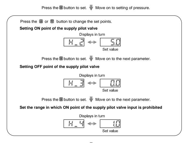
Press the S button to set.  $\P$  Return to function selection mode.
