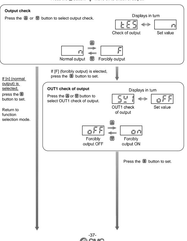
Press the S button.  $\P$  Move on to check of output.
