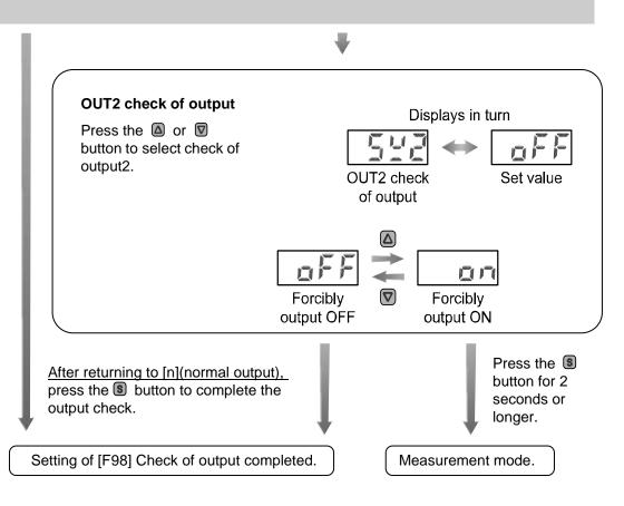
\*: Return to measurement mode from any point by pressing the S button for 2 seconds or longer.
