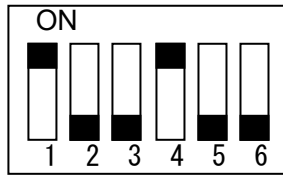
(b) Open collector input (5V)
