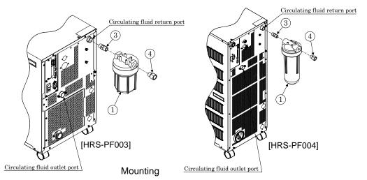
[Materials of wetted parts] Stainless Steel, PTFE, PP, Acrylonitrile-styrene, NBR (PE: Element)
