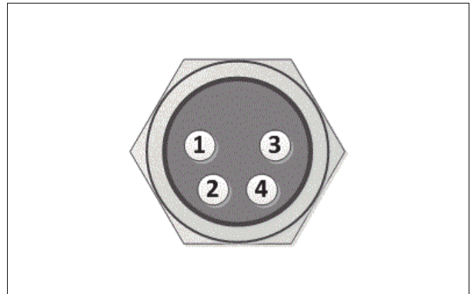
Fig. 14 Pin assignment in female connector view (connector in device)
